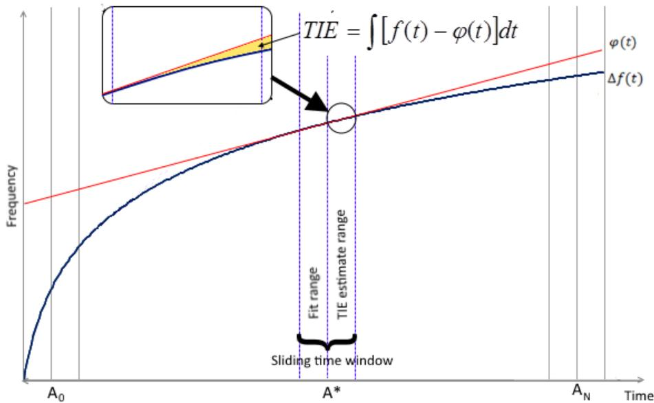
Fig.1 TIE estimation algorithm.
