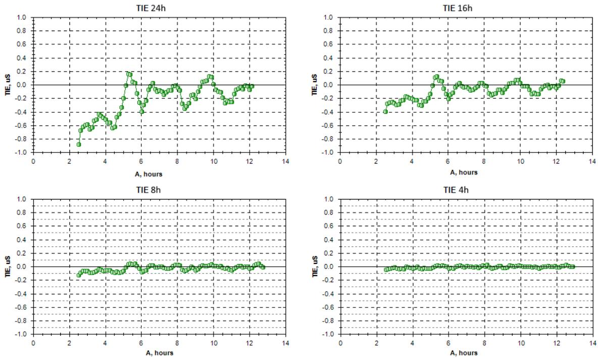
Fig. 7 Measurement of TIE per 4, 8, 16 and 24 hours
