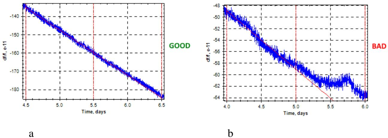
Fig.5 Figure 5a aging curve satisfactory for TIE of 100...400 ns requirement. Figure 5b shows “standard” aging curve.
